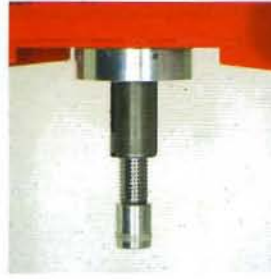
Manual screw extension for quick approach and fine adjustment.
